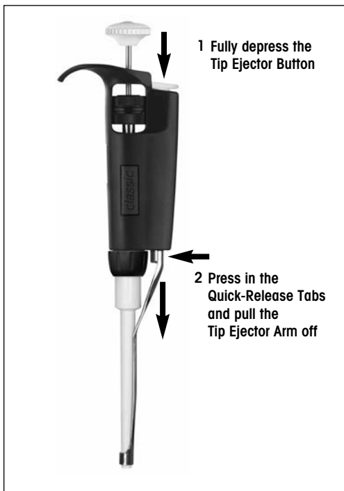
Figure 3 Removing the Tip Ejector Arm
